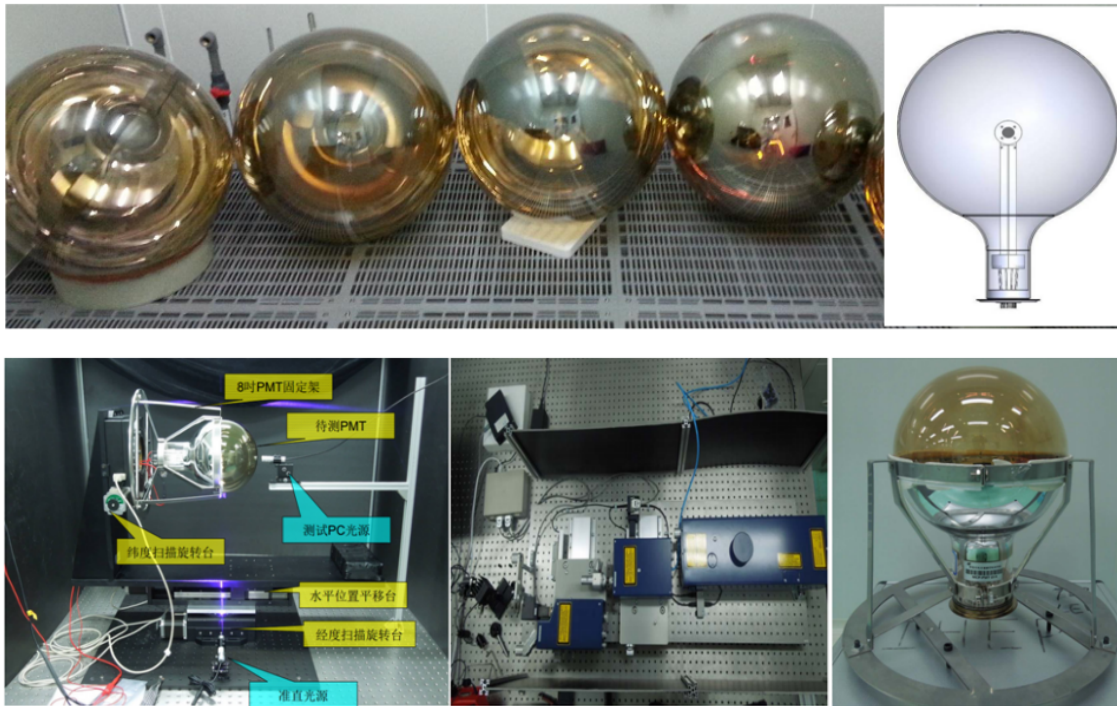
Figure 4.6: Various 20" PMTs under test, and PMT testing systems set up in IHEP, Beijing; from [62].
